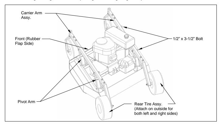
Figure 2: Carrier Arm Installation
